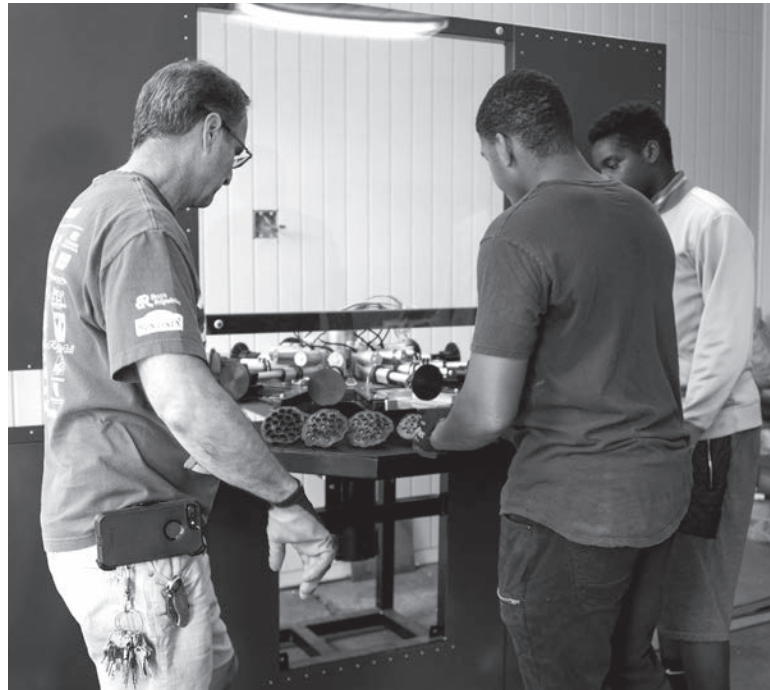
MODERNIZING THE PROCESS: Wreath production supervisor John Lemieux shows two Boys Republic students how the new semi-automated pod cutter functions. The machine, designed by Cal Poly Pomona Engineering students, is six times more effective than the manual process of cutting lotus pods that adorn Della Robbia wreaths.
